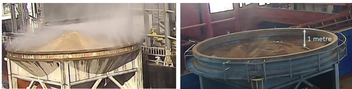
Figure 5.5: Left: Maximum fill height for hopper with grizzly. Note this picture shows a hopper with misting sprays. Misting spray are no longer in use. Right: Maximum fill height for hopper without grizzly.
