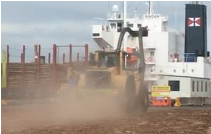
Figure 1. Example of excessive visible airborne dust.
