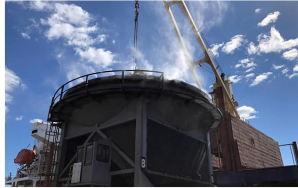
Bulk hopper water misting
